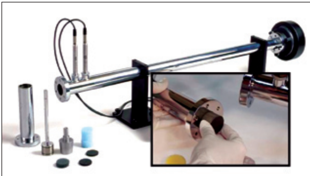
Figure 13. Impedance tube used for measuring transfer impedance (from Spectronics, Inc.).
